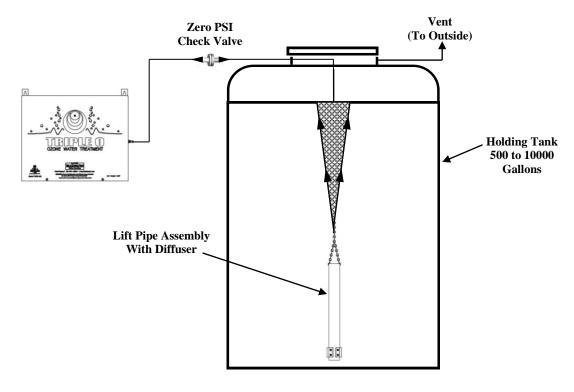
**Model RO-TWTS** is specifically designed for RO product water stored in an atmospheric holding tank. It controls bacteria, raises pH into 7-7.5 range and adds dissolved oxygen. It is designed to operate 24 hours per day or can be time clock operated if desired.
