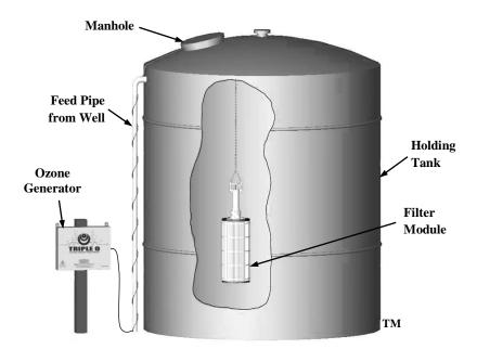
The Triple O system consists of an ozone generator with an air pump and filter module (with 100 square feet of filter area) that hangs inside the tank and includes an ozone diffuser to create millions of ozone saturated bubbles. An optional in-line mixing system (installed on the well feed line to the water tank) is also available.
